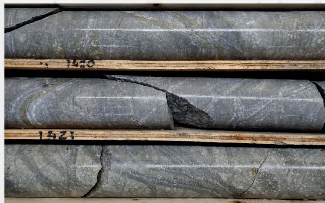
419-421 m Crowded porphyry, intense py D veins with sericite envelopes (pyrite halo)
